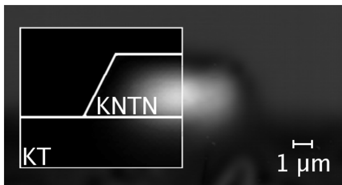
Figure 4.5: Waveguide profile and TE mode intensity distribution of \lambda = 1579 nm laser light propagating in a potassium sodium niobate tantalate thin film ridge waveguide. Left inset shows simulated mode profile with excellent agreement to measurement.
